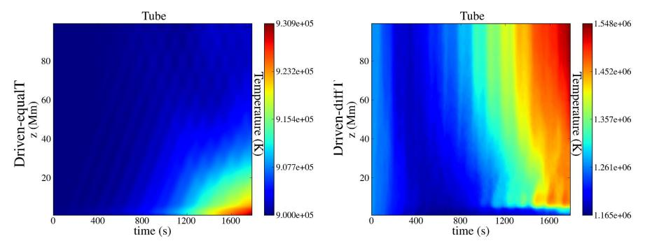
Time – height plot for the average temperature for the two models with the footpoint driver. We focus only on the flux tube (for density  $\rho \ge 0.335 \rho_i$ ).
